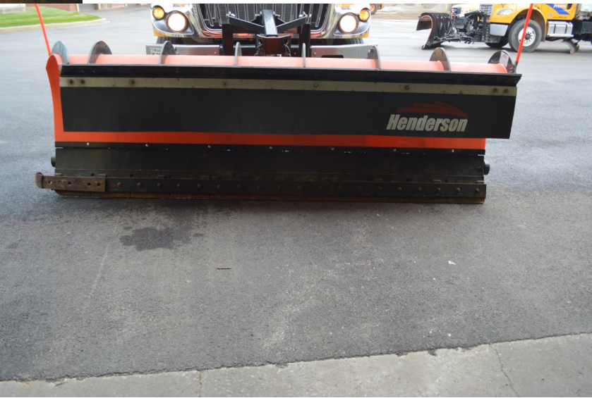
The new style sectional blade contours the pavement much better, leaving a cleaner plowed surface.
