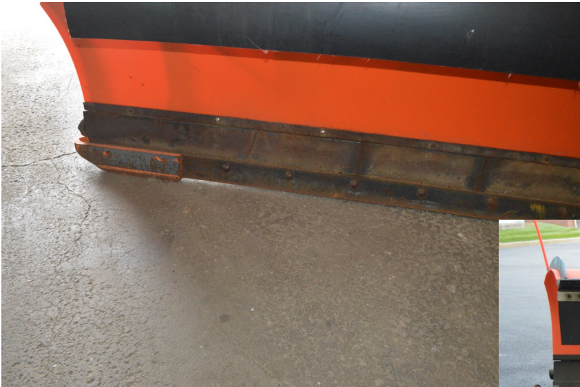
This is an old mild steel set up, showing the uneven wear causing a trailing of snow condition and sub optimal driving conditions.
