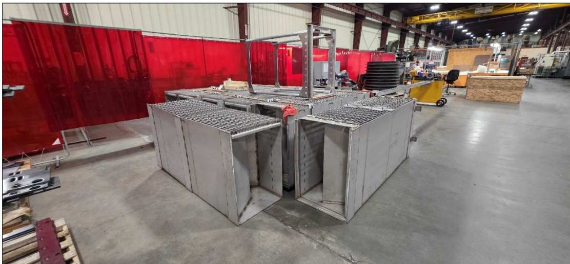
Plate 1. Finished sections at the fabricator’s establishment. Note the capture net framework on top of the segments.
