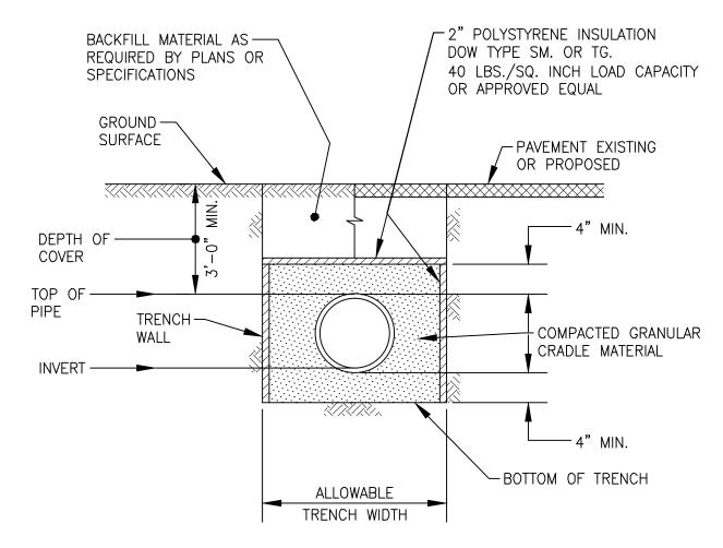
REQUIRED WHEREVER DEPTH OF COVER IS LESS THAN FOUR (4) FEET FOR BUILDING SERVICE SEWERS AND IS LESS THAN FOUR (4) FEET FOR MAIN SEWERS. DEPTH OF COVER IS MEASURED OVER TOP OF PIPE AS INDICATED ON THE ABOVE DETAIL.
